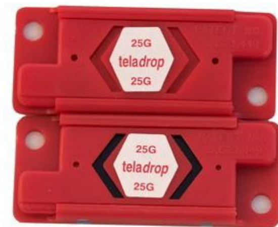
Figure 1: The dark arrows on the shock-watch indicate the package experienced excessive shock during shipping. Red arrows indicate no shock above the G level indicated.
