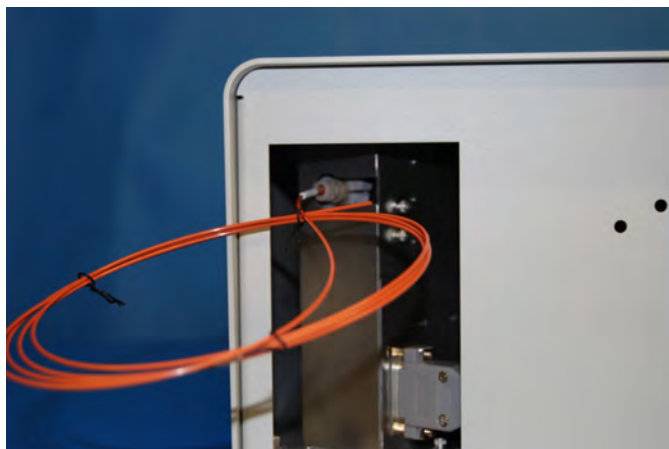
Figure 19: Photo of the back of the Auto-collector needle assembly and location of the union fitting to connect the PEEK tubing from the PILS peristaltic pump.
