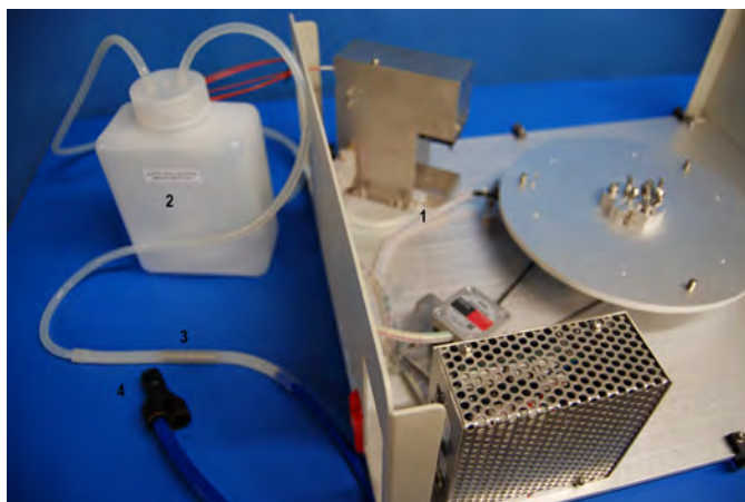
Figure 20: Photo of the Auto-collector drain bottle.
