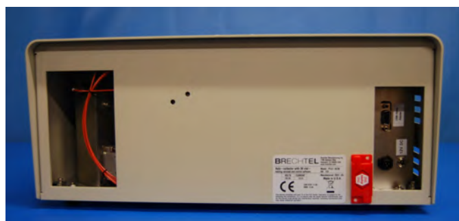
Figure 12: Photo of the back of the Auto-collector showing the liquid sample supply connection at the rear of the needle assembly (to the left), and the serial communications and power hookups to the right.
