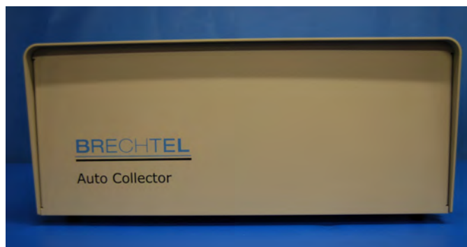
Figure 11: Front of the Auto-collector with all covers installed.
