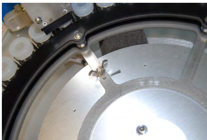
Figure 25: Photo of a properly installed vial-holding carousel.
