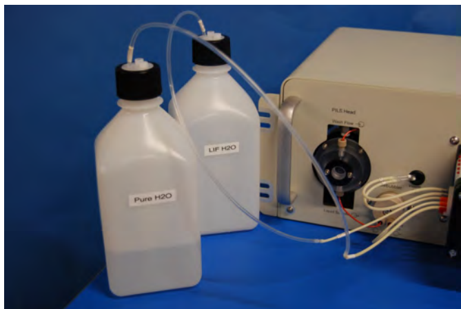
Figure 10: Washflow and Steam Liquid Flow (pure H 2 O) water supply bottles.
