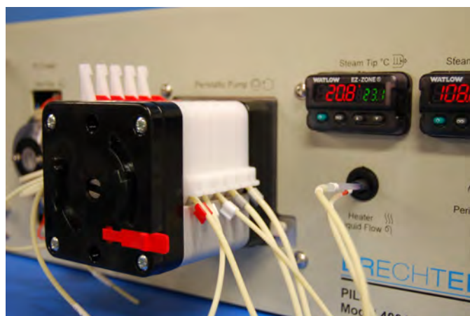
Figure 8: View of flow output side of the peristaltic pump.
