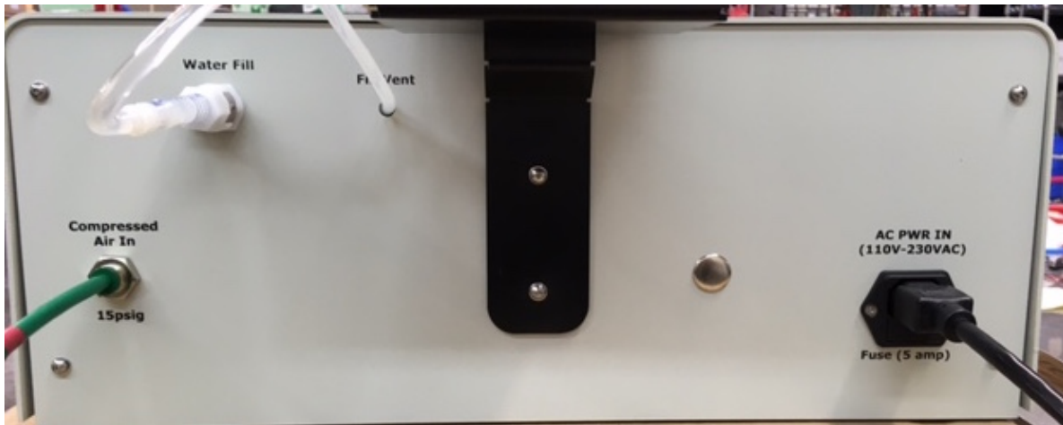
Figure 4: Rear view of the Pre-Humidifier chassis.
