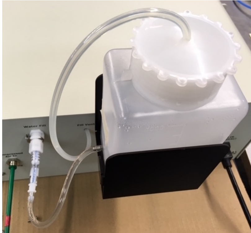
Figure 3: View of the Pre-Humidifier Water Fill Bottle mounted to rear panel of chassis.
