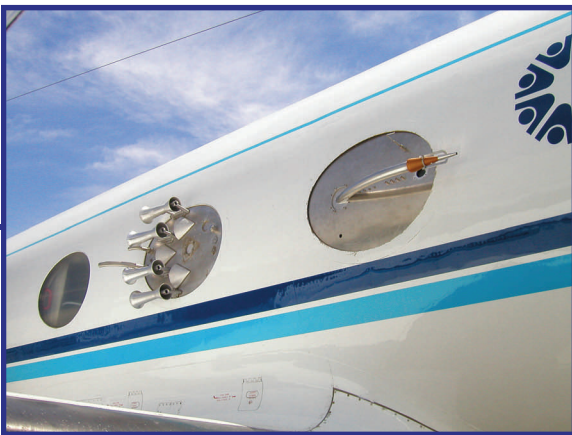
Inlet System Model 1200 installed on a research aircraft
